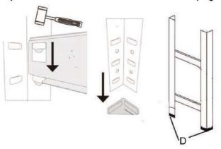
**2.** Assemble end frames with short side beams and add long front and back beams to join the frames together.
