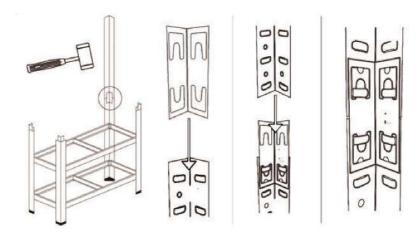
**5.** Repeat steps 2 and 3 to add the remaining levels. Insert MDF boards at an angle, corners first.
