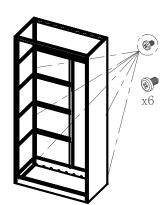
4. Install G into body of cabinet fix by screws
