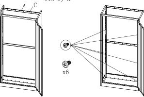
5. Install I into body of cabinet, as shown in the following figure
